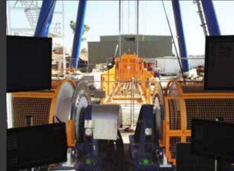
The system utilises a SIL 3 Capable ABB AC500-S PLC platform, providing system control and safety monitoring. All safety devices have been designed to meet or exceed the requirements of MDG2005 and have been independently certified as meeting relevant functional safety requirements, for example SIL 2. The system layout and associated programming is fully customised for each installation and is tailored specific to the project, such as additional gate monitoring and pipe handling modes.
